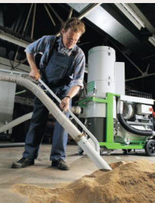
Bulk spillage collection with aeration tool
