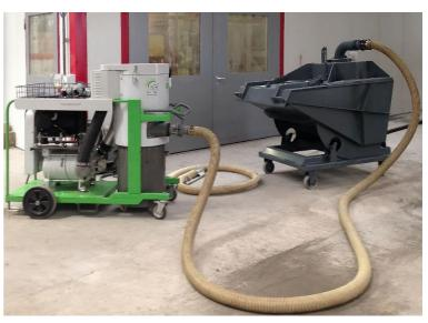
Hoses and tools are available in 51mm, 76mm and 102mm sizes. Ti80 is suitable for multiple operators and also fixed pipework installations. A skip interceptor is available as an option.
