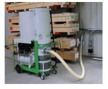
Displaced air is filtered within the BVC 'clear flow' filtration system and particles are collected within a removable bin at the base of the unit. This is equipped with a bin balance arrangement for use with plastic liners. The bin is provided with a 'lift and tip' forklift attachment to ease the transportation of the full bin and discharging the sealed bag for onward disposal.
