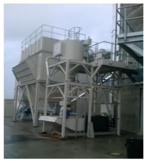
An inclined conveyor gantry, approximately 240m long, moving the material from the intake enclosures to the storage silo. One system serves a lower section of the conveyor together with two lorry intake stations interconnecting 9 hose connection points fixed to a vacuum plant. A second system serving the upper section of the conveyor, including silo penthouse and platforms / plant beneath, interconnecting 11 hose connection points fixed to a vacuum plant.
