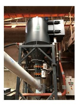
The extracted products, which are mainly powders and small granulate are separated from the conveying air within a filter separator, having filtration media cleaned by the reverse jet technique. The materials are dispensed through a double dump valve system into a screw conveyor for onward processing.
