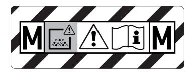
**M**: (MEDIUM HAZARD) suitable for separating dust with a limit value of occupational exposure greater than 0,1 mg/m<sup>3</sup>
